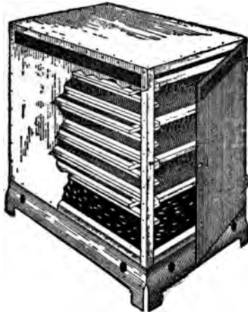
FIG. 8. Home-made drier of galvanized iron, for use on stove.
